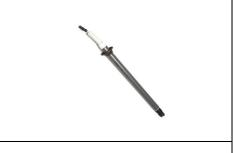
Suction lance WITHOUT LEVEL PROBE 8x12 45cm -pre assembled PVC/PP suction lance with foot filter (to avoid the pump sucks suspended particles) and suction valve (to avoid the suction tube's emptying)
